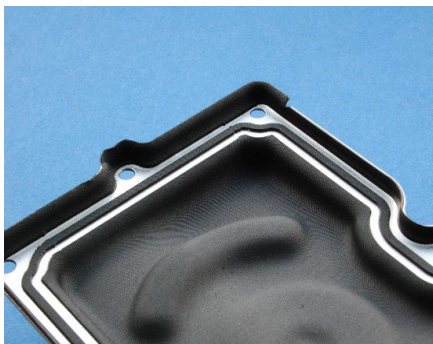
Sealing pre-treatment of an aluminum housing
