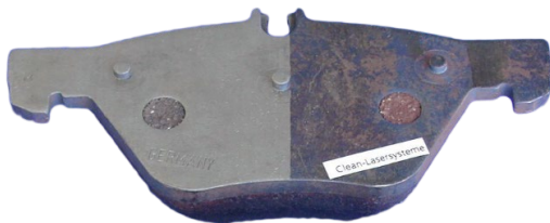
Partially laser pre-treated brake pad (unit price approx. 1 cent per component)
