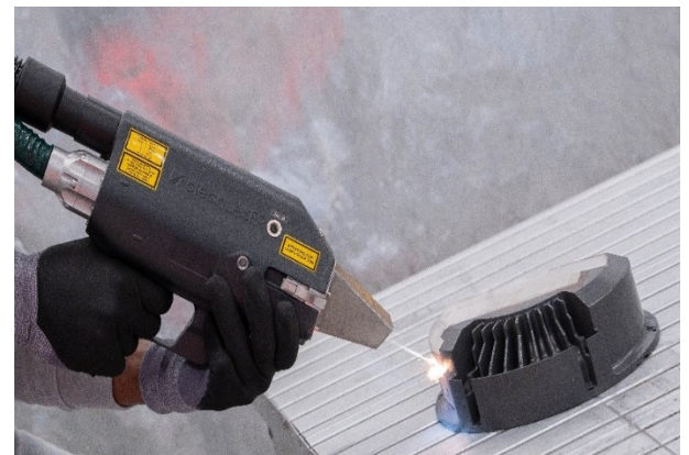
Suitable optics for homogeneous distribution of the laser beam
