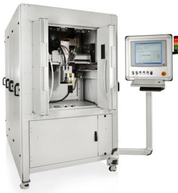
Modular laser machine cleanCELL with manually opening front door
