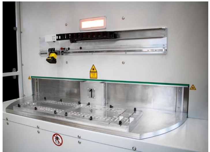
cleanCELL with rotation table for main cycle time parallel (un-)loading
