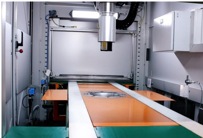
tireCLEANER: Processing area with turnMOTION optics and conveyor technology
