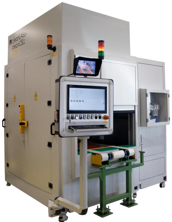
tireCLEANER: cleanCELL 3220 with conveyor belt extension for integration into an interlinked operation
