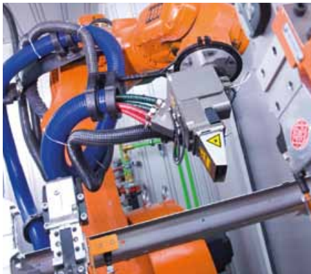
cleanLASER when welding in car body pre-treatment
